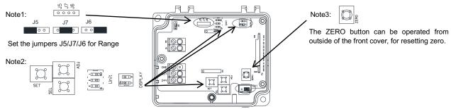
1. Unit setting: Set the unit switch as below.
